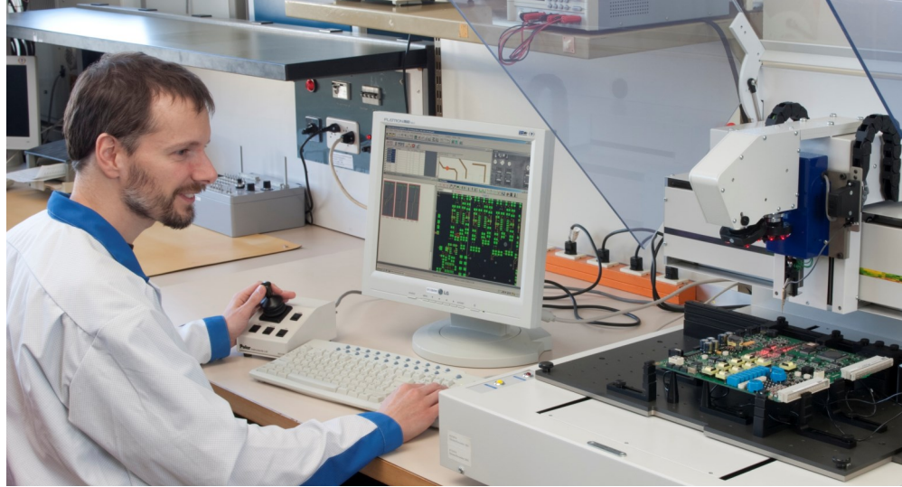
FIGURE 1 — EXAMPLE OF A SIGNATURE ANALYSIS TESTING SETUP WITH THE NFF DEVICE UNDER TEST ON THE RIGHT-HAND SIDE.
